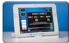
Figure 2. Monitor display showing change in pulse rate, pulse strength, pulse irregularity, and oxygen saturation, pulse rate, and an Alert Level 3.
